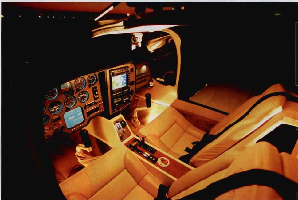
The Liberty XL2's engine is simple to operate—just flip a switch on the center console and the FADEC system handles the rest. Add the optional Garmin avionics suite, and you've got 21st-century situational awareness.
