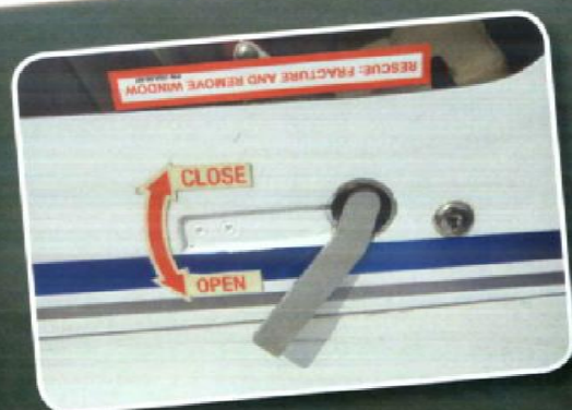
Neat, recessed door latches work perfectly and minimise drag. Rescue instructions cover escape from inverted – roll-over hoop protects occupants
