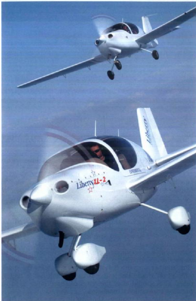
The Liberty XL-2 is a new two-seat touring aircraft designed to meet the needs of the private owner/pilot. It features a chromoly welded steel rolling chassis and a carbon fibre fuselage.
