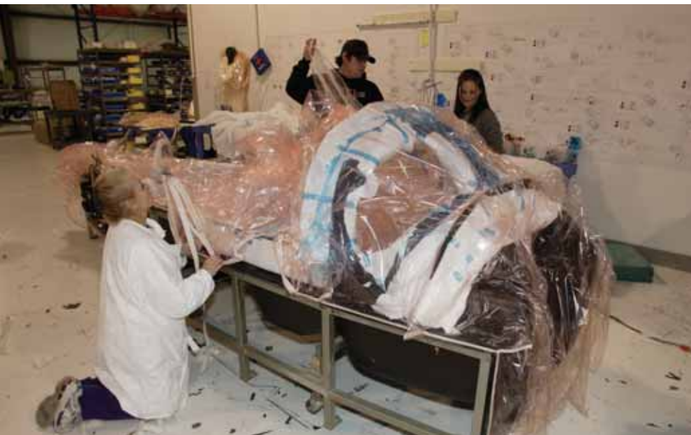
Samantha Jay (background), team leader for the lower half of the Liberty fuselage, prepares a carbon fiber shell for fittings.
