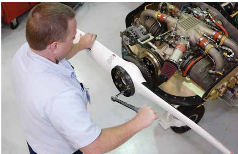
Liberty's Phil Lindstrand re-torques and re-wires the bolts on the composite propeller of the Liberty XL2, something the Cessna 172's metal propeller does not require.
