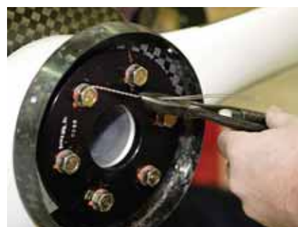
Liberty's Phil Lindstrand re-torques and re-wires the bolts on the composite propeller of the Liberty XL2, something the Cessna 172's metal propeller does not require.
