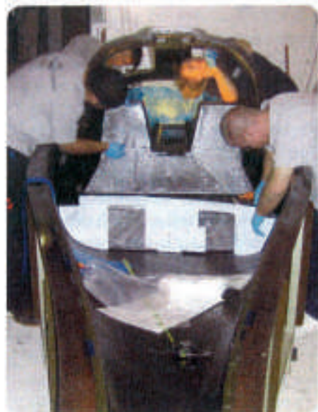
Workers at Liberty Aerospace lay prepreg carbon reinforcements into the mold.
