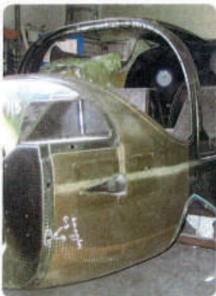
Molded Fuselage for the LX2 after being oven cured. When trimmed the part weighs between 101 and 103 lbs.
