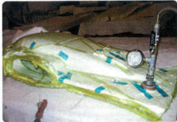
Wheel Fairing being vacuum bagged using the glove bag technique.
